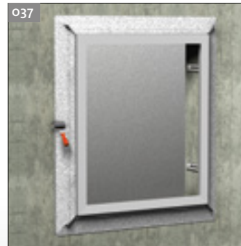
037 Press the strip into the adhesive bed.
