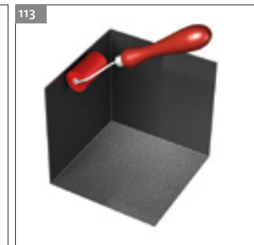
113 Roll over the bonded surface with a hard rubber roller.
