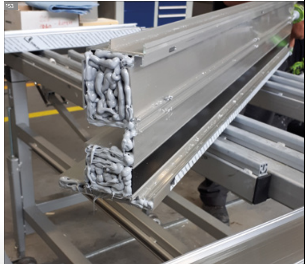
Bonding of metal section ends with TEROSON SE 2000 MF
