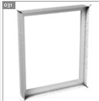
o31 Window frame with all-around sealing strip incl. loops formed in the corners
