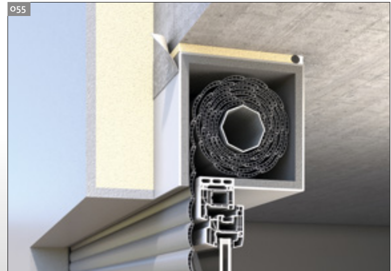
055 Sealing with TEROSON FO 1 FOIL-TACK on the outside
