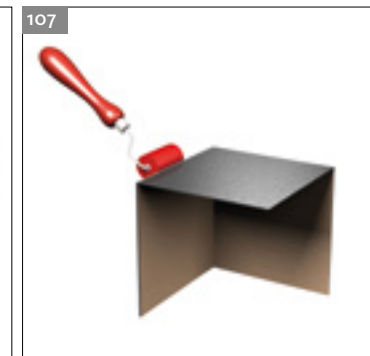
107 Roll over the bonded surfaces with a hard rubber roller.
