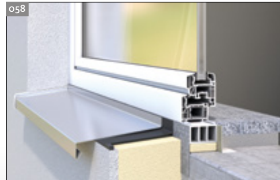
ETIC system: 2nd sealing layer produced with TEROSON FO 3, PT ecoMAX 600 and SK1
