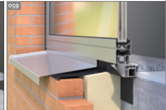
Clinker facade: 2nd sealing layer produced with TEROSON FO 3, PT ecoMAX 600 and SK1
