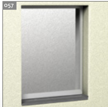
Window element with windowsill installed
