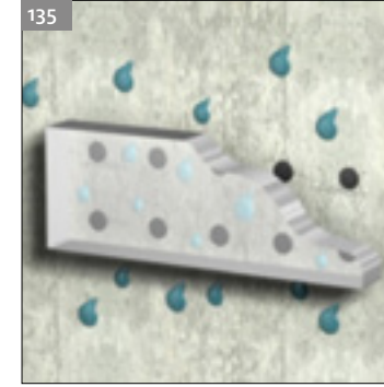
135 Spot application: moisture cannot accumulate.
