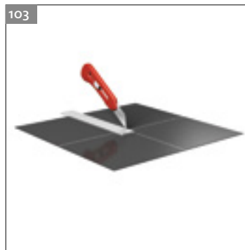
103 Cut along the marked lines with a cutter knife.
