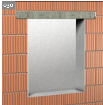
o30 Window opening with smooth trowel finish
